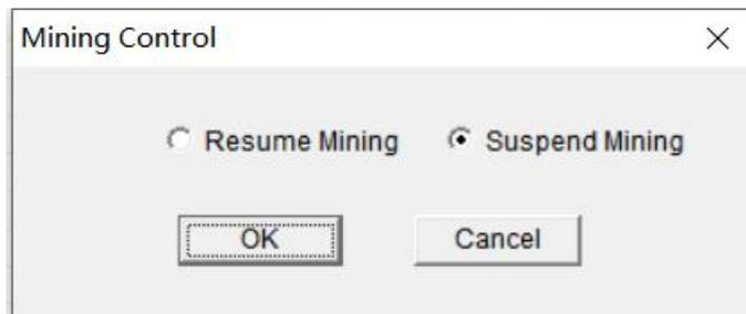
After the selection, a pop-up window will pop up to choose to resume mining and stop mining. Select one and press OK to switch the mining mode.
